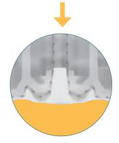
When touching the adhesive the remaining air is evacuated making sure the adhesives stays retained.
