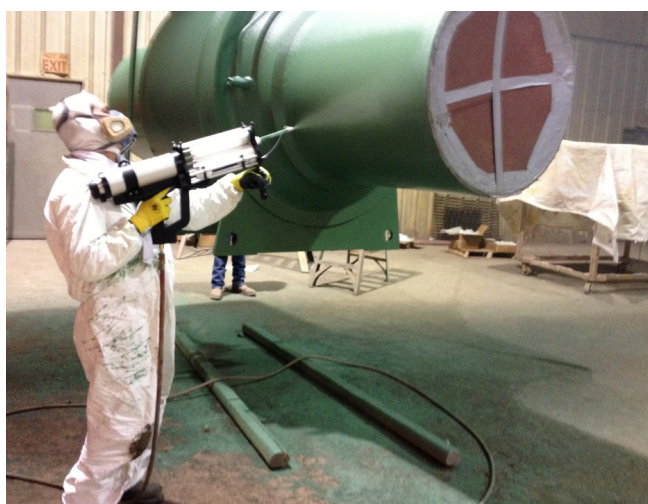
Figure 2. Spray application of a 36 in. ball valve.
