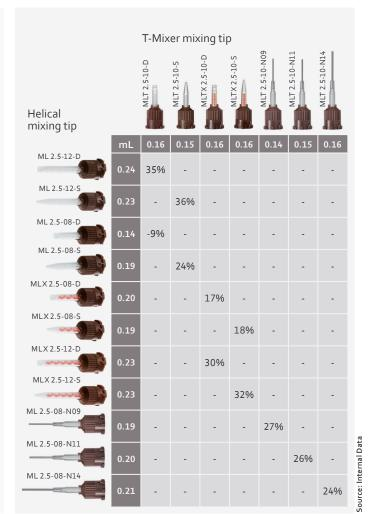
mL Waste volume in milliliters (mL) for the T-Mixer and Helical mixing tips.
