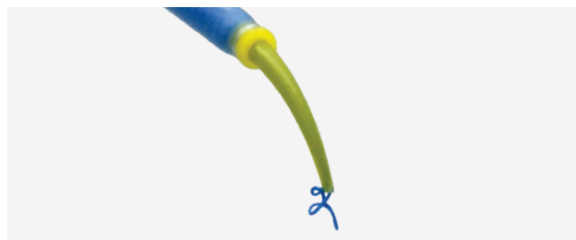
Inconsistent material flow (spiral jet) caused by a burr defect at the outlet of the Intra Oral Tip.
