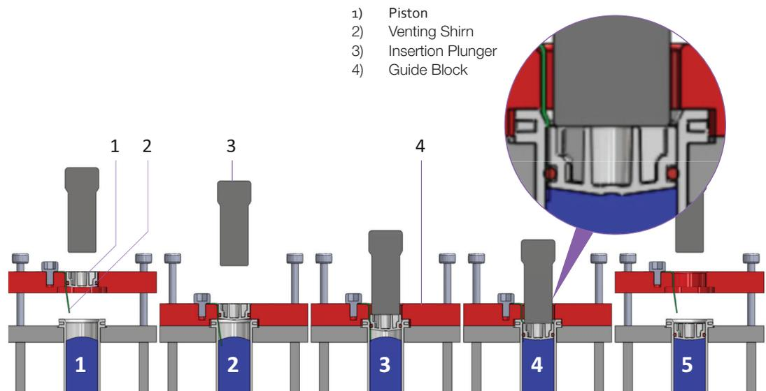
1. Install cartridge into a properly designed guide block and then place piston into said block so that its rib structure can be seen from the top. The piston should fit down into the block and be square with the cartridge.
