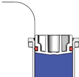
Do not overfill the cartridge as it may leak and/or not fit into the dispensing tool.
