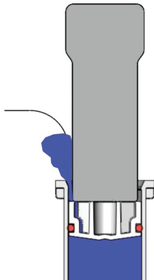
In this scenario the plunger pushes too long and/or with too much force on the material such that it pushes up beyond the O-ring seal. Some fillings will tolerate small amounts of material getting past the seal but others will not.
