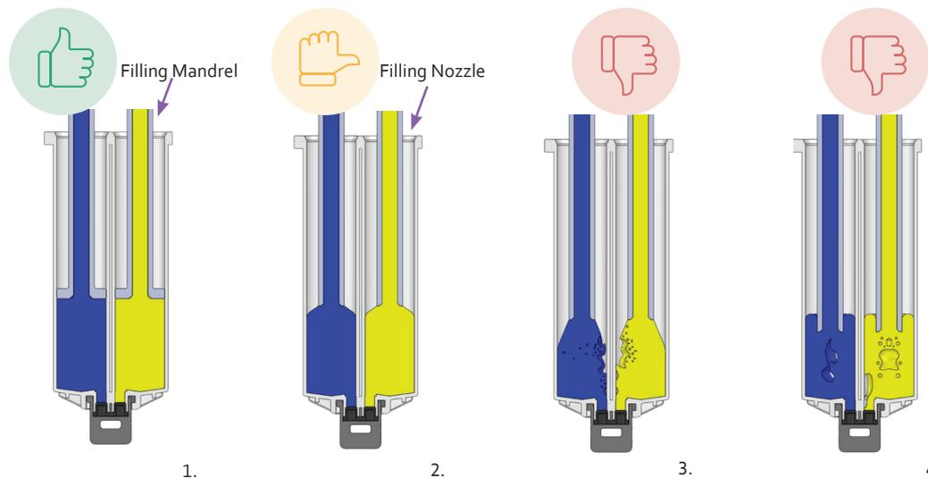
1. A properly made filling mandrel fits tightly to the inner diameter of the cartridge and provides the most effective means of filling. It allows a small amount of air to escape from the side. The material is pumped through the mandrel and the cartridge is pushed off the mandrel. In this scenario it is easy to add a limit switch to control the filling height. Additionally, it takes the control away from the operator as you will see in scenarios below.
