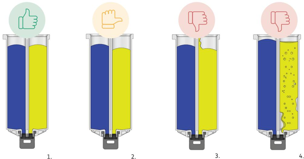
1. Both of the filling levels in the first scenario are equal, there is no air trapped within the material and the profile at the top of both A- and B-sides filling is slightly domed upwards.
