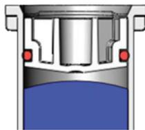
This scenario shows that the piston has been inserted into the cartridge such that not all air was allowed to escape from underneath the piston. This cartridge will likely not meter accurately leading to poor performance of the two component material. See also "Multicomponent systems - Effects of air inclusion"
