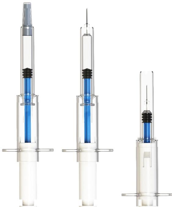
*Figure 1: SicuroJect before use with needle cap (left), before use without needle cap (middle) and after use (right), after the safety feature has been automatically activated and the needle has been retracted*
