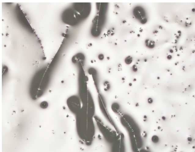
Fig. 5 Zirconia sample treated with conventional fiber-flocked micro applicator (Primer A)
